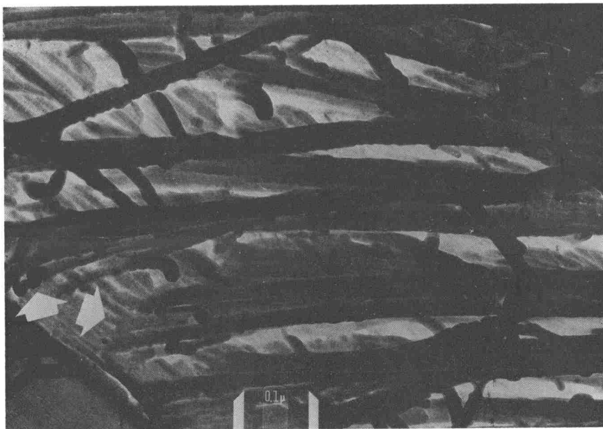
Fig. 7. Carbon replica showing inner core fiber bundles. Electron micrograph.
