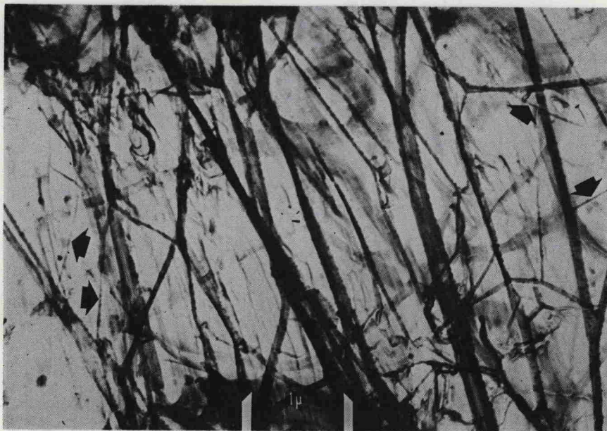
Fig. 8. Microtomed, \text{Br}_2 -stained section from the inner core. Transmission electron micrograph.
